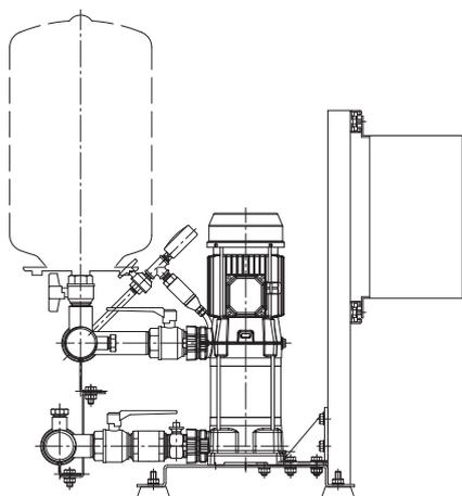
Inverter-controlled units with two vertical multistage pumps.
